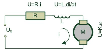
Fig. 2 Equivalent circuit of motor
