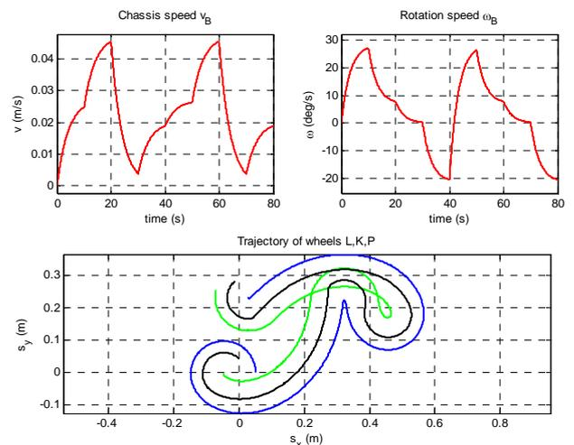
Fig. 11 Dynamic behaviour - periodic voltages – speeds and trajectories
