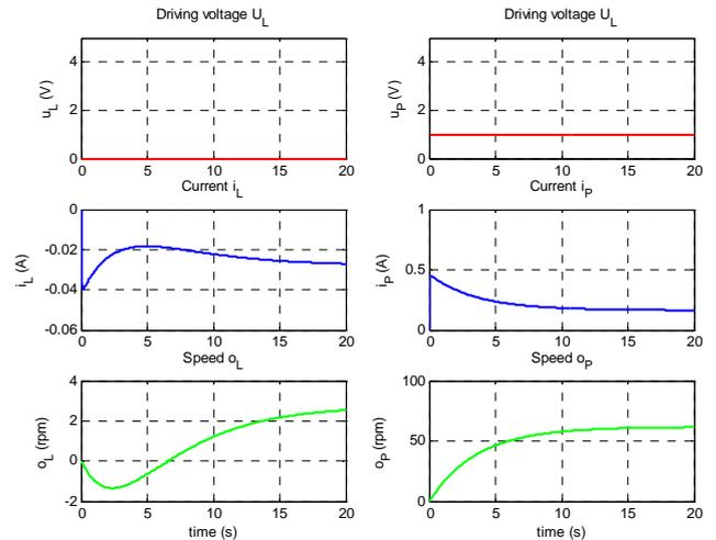
Fig. 9 Dynamic behaviour - constant supply voltage 1 V for right motor
