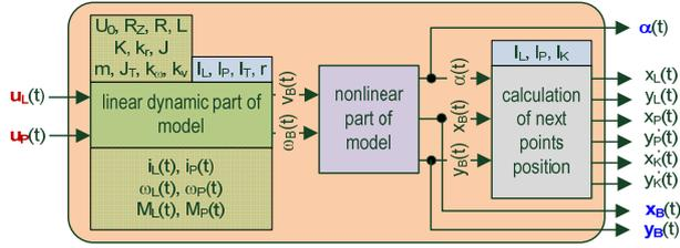
Fig. 7 Model partitioning into linear and nonlinear part
