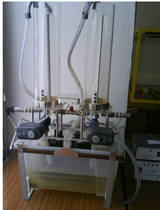
Fig.2 Two tanks process
